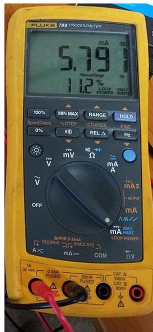
Figure 3. Loop Resistor enabled in Loop Calibrator
