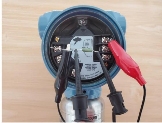
Figure 2. Correct Loop Resistor Connection
