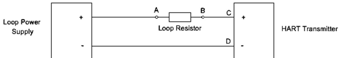
Figure 1. Loop Resistor Placement in the Loop
