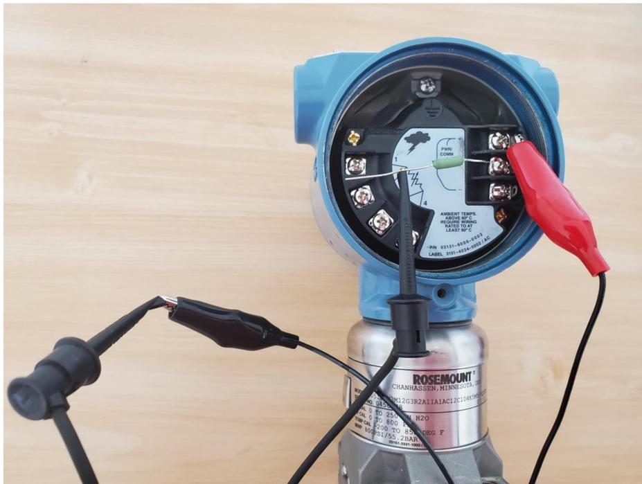
Figure 4. Wrong! Modem in Series with Loop Power
