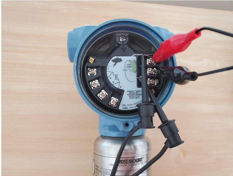
Figure 5. Wrong! Loop Resistor Across Device Input Connections
