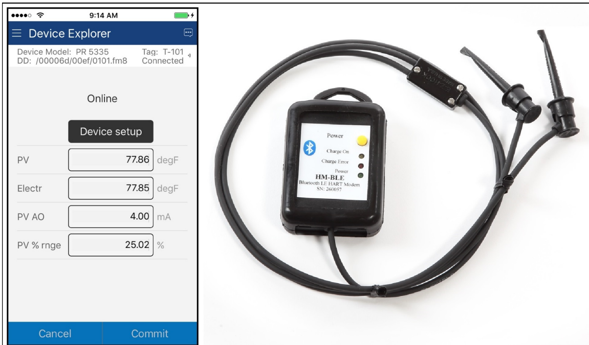
DevCom.iOS HART App + HM-BLE Bluetooth Low Energy HART Modem
