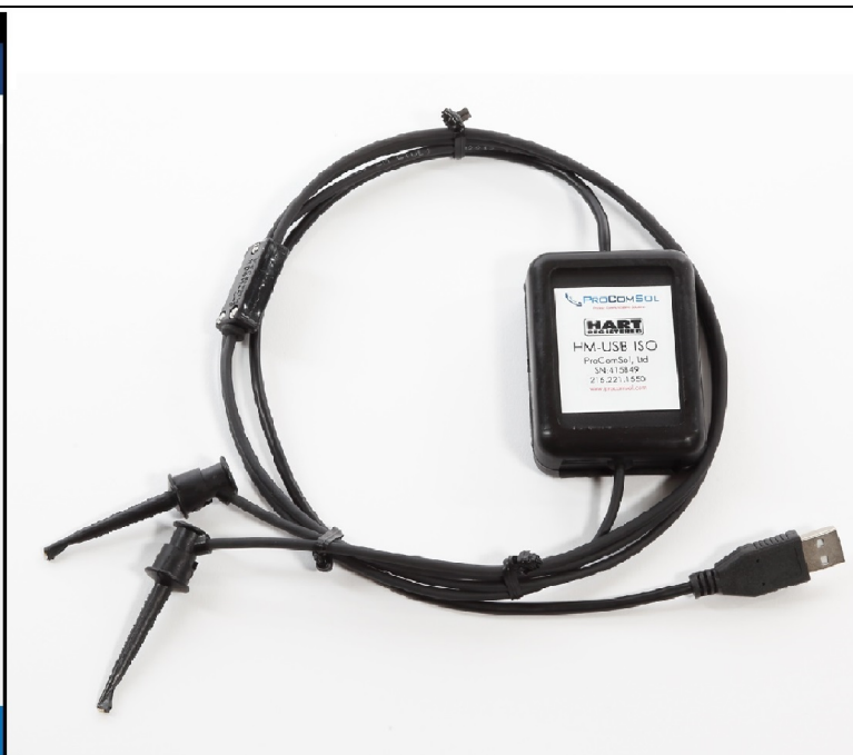
DevComDroid HART App + HM-USB-ISO HART Modem
